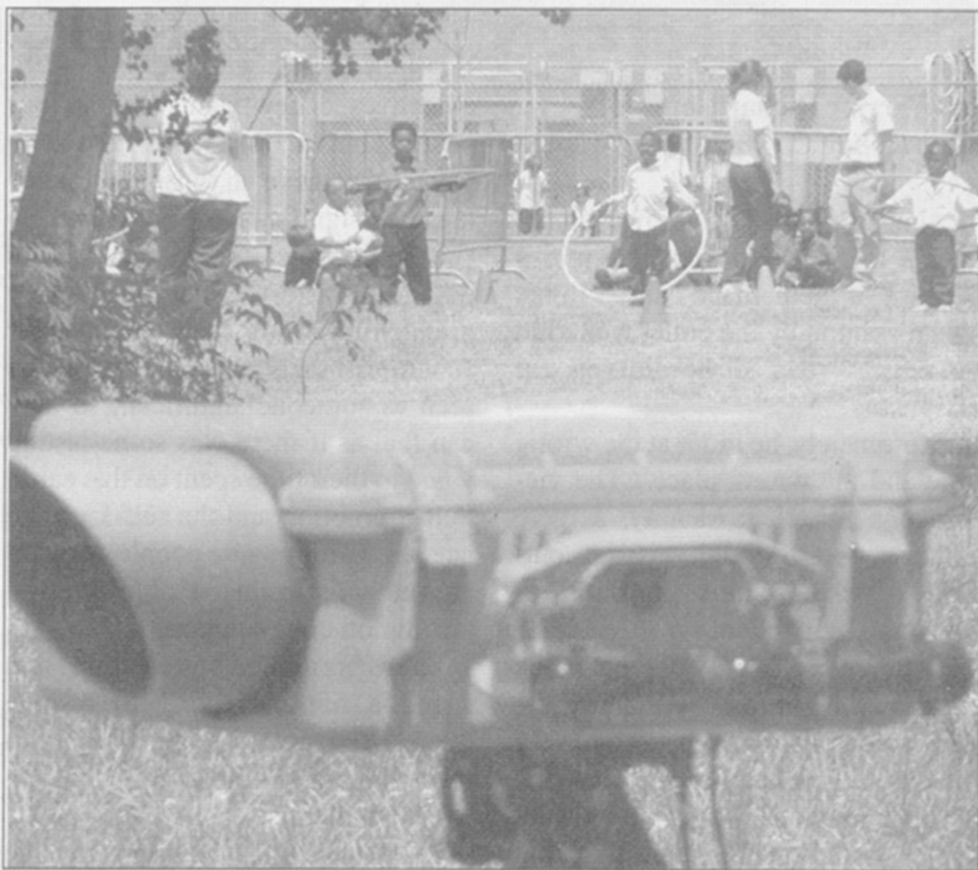
This open-air monitor will test and process air for six known carcinogens 24 hours a day, giving Louisiana environmentalists a new weapon in the fight to clean up the air, land and water.
